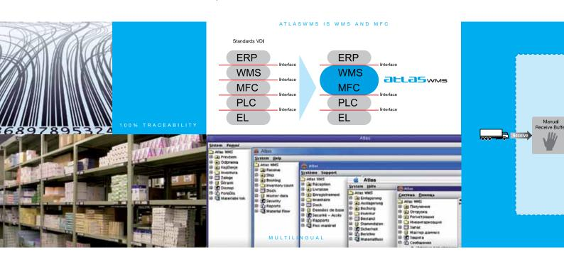
As an MFC (Material Flow Control) it coordinates the automatic transport devices (stacker cranes, carousels, conveyors, etc.).
