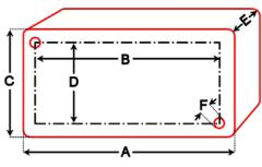
A = 125mm B = 113mm C = 80mm D = 52mm E = 57mm F = 4mm
