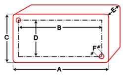
A = 98mm B = 86mm C = 64mm D = 36mm E = 36mm F = 4mm
