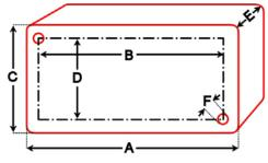
A = 220mm B = 204mm C = 120mm D = 82mm E = 81mm F = 6mm
