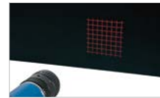
Grid 0.05 mm line thickness.
