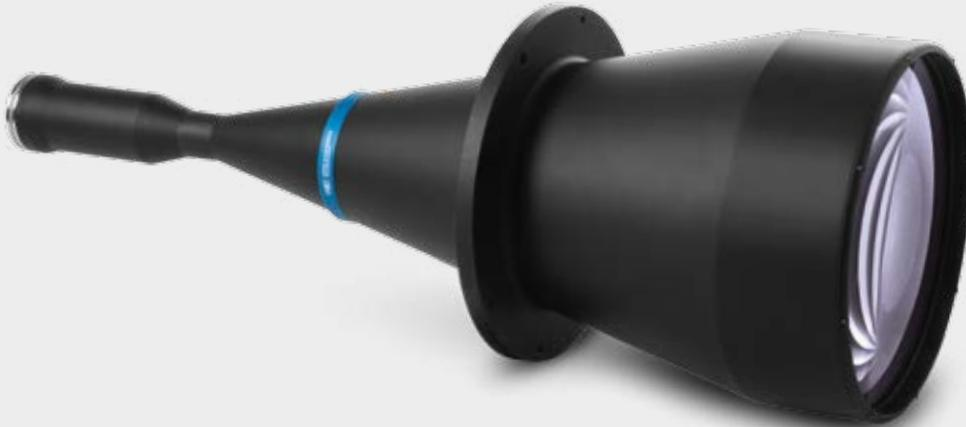
**TC16M series** telecentric lenses have been specifically designed to fit 35 mm format (36 x 24 mm) detectors with very high resolution, such as 11, 16 or 29 Mpix. This combination is the typical choice for extremely accurate measurement of large items such as engine parts, glass or metal sheets, PCBs and electronic components, LCDs, etc.
