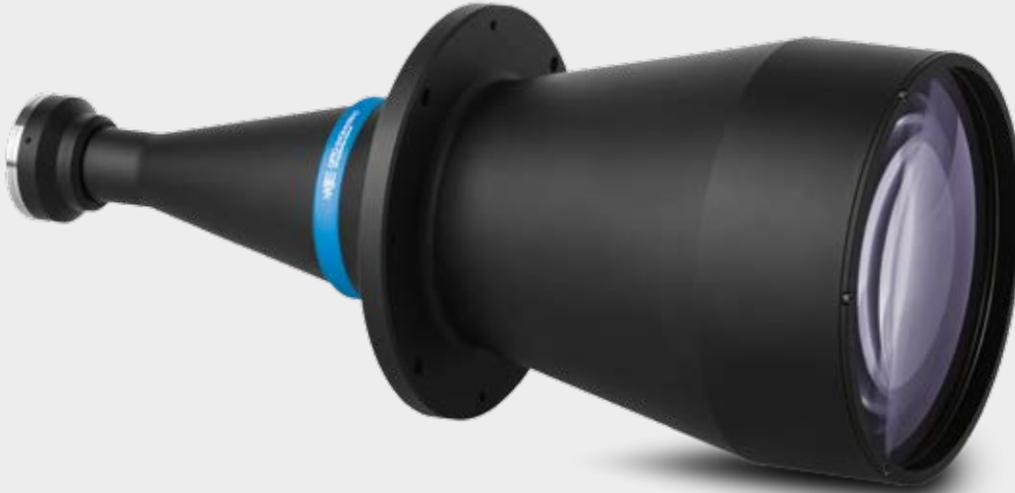
**TC2MHR and TC4MHR series** are high resolution telecentric lenses designed for detectors larger than 2/3": TC2MHR lenses cover up to 1" detectors (16 mm diagonal) while TC4MHR lenses cover up to 21.5 mm detector diagonal (e.g. suitable for 4/3" detectors), making them the perfect choice for advanced metrology applications.
