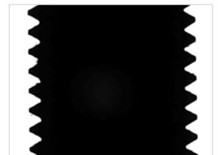
A TCLWD050 lens assembled with a CMHO016 clamping mechanics and back-illuminated by a LTCLHP016-G telecentric illuminator forming an inspection system for measurement of mechanical components such as milling tools and screws.
