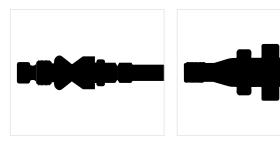
Engine shaft measurement performed with TC4K lens coupled to LTCL4K telecentric illuminator by means of two CMMR4K deflecting mirrors.
